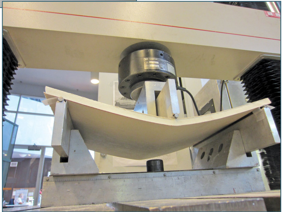
Photo 5 – Flexural test in progress.
